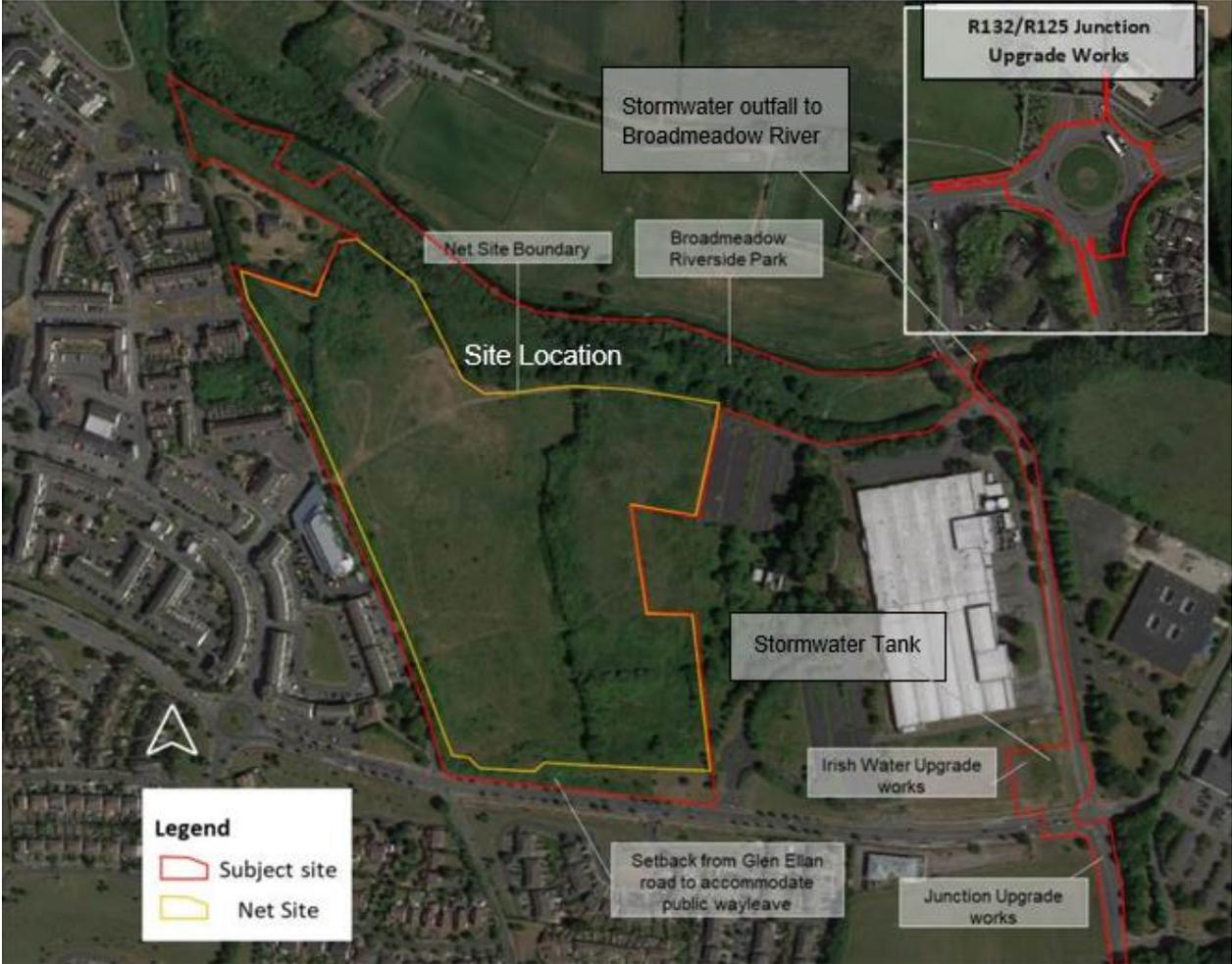
The site generally falls from south to north towards the Broadmeadow River. The ground levels to the southwest are in the order of 14.0m falling to 5.6m at the northeast. See Figure 3 below illustrating the existing ground contours.
